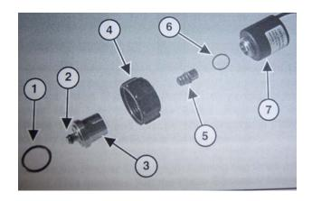
After extended use the soft plunger seal (Item 1) will wear a groove where the seal impacts the hard orifice seat. Replace plunger if worn or damaged.
