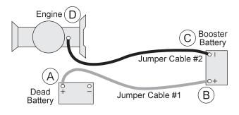
To prevent damage to other electrical components on unit being started, make certain that engine is at idle speed before disconnecting jumper cables.
