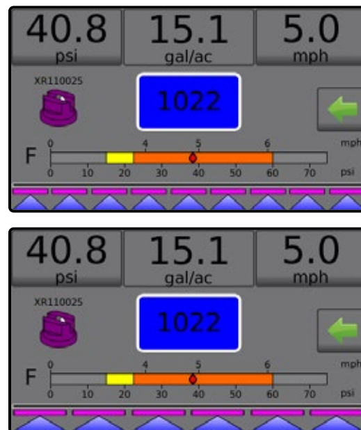
Figure 3-41: Operation Screen with 9 or 6 Sections
