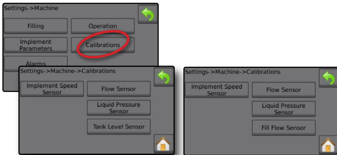
Figure 3-15: Calibrations – Tank Level Sensor and Fill Flow Sensor
