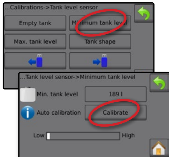
Figure 3-30: Tank level sensor – Minimum tank level
