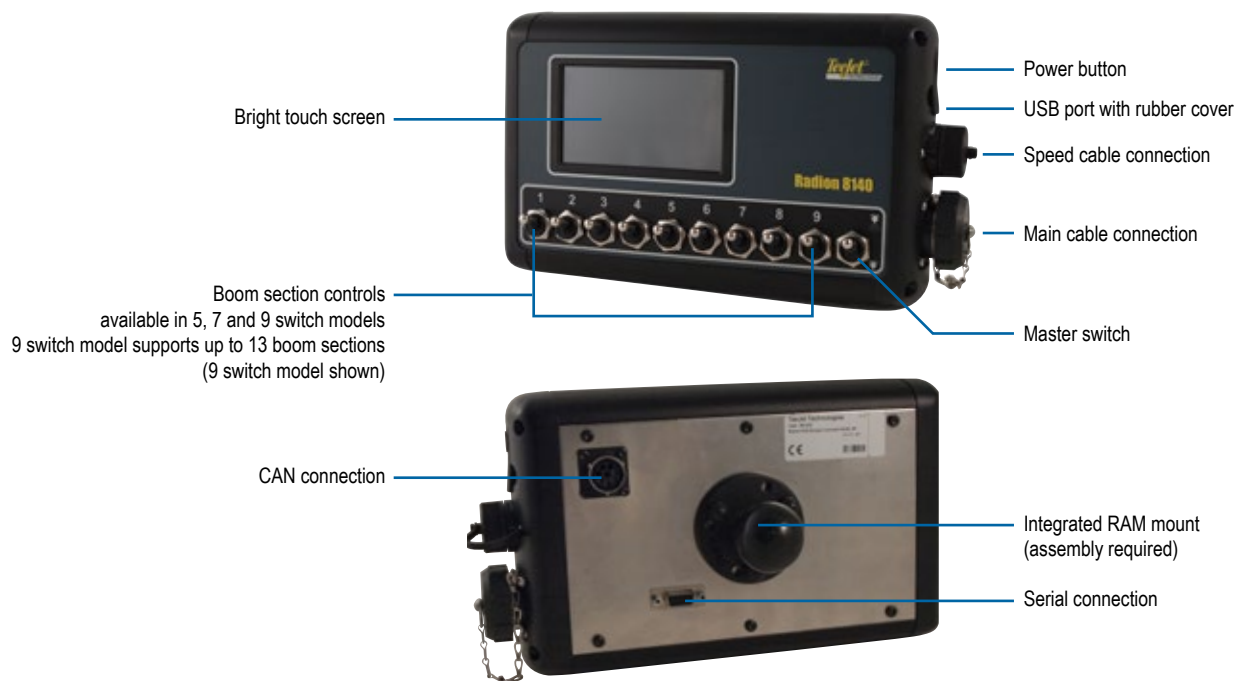
Figure 1-1: Radion 8140 console front and back
