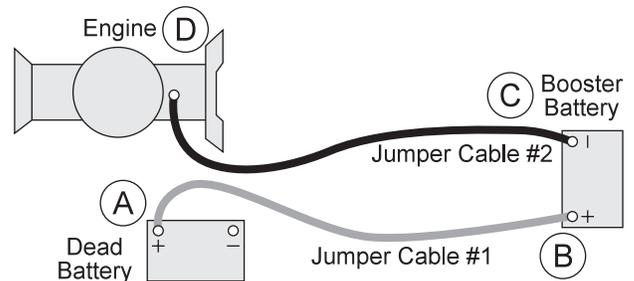
To prevent damage to other electrical components on unit being started, make certain that engine is at idle speed before disconnecting jumper cables.
