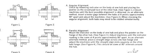
Securely tighten foundation bolts and recheck the alignment. Adjust the machines again, if necessary.
