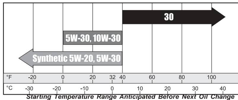
Air cooled engine run hotter than automotive engines. Use of multi-viscosity oils (10W-30, etc.) above 40° F (4° C) will result in high oil consumption and possible engine damage. Check oil level more frequently if using these types of oils.
