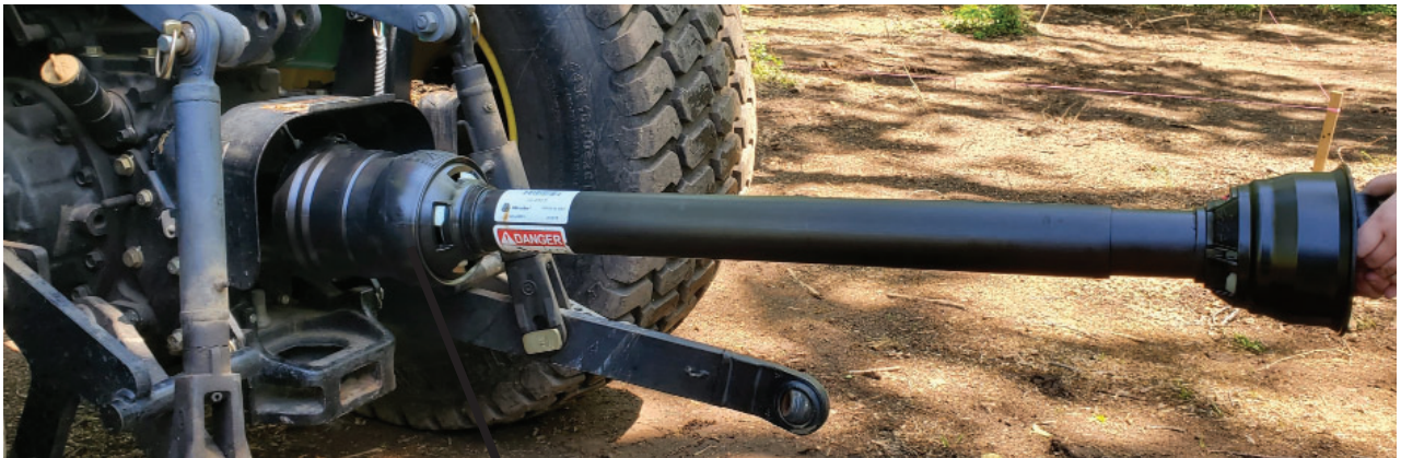
PTO connection with larger guard housing goes to the tractor.
