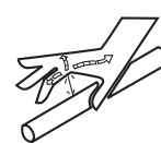
Hydraulic Fluid Penetration
