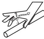
Hydraulic Fluid Penetration
