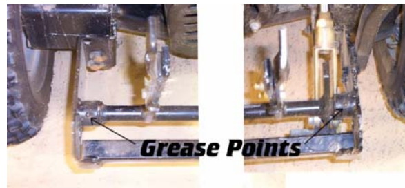
Rake Lift Grease Points
