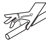
Hydraulic Fluid Penetration
