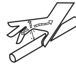
Hydraulic Fluid Penetration
