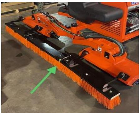
**Step 8.** Install the right side brush using the (4) 5/16" x 1 bolts and tighten.
