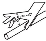
Hydraulic Fluid Penetration
