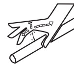
Hydraulic Fluid Penetration
