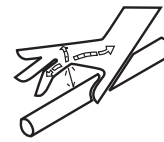
Hydraulic Fluid Penetration
