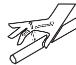
Hydraulic Fluid Penetration
