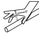
Hydraulic Fluid Penetration
