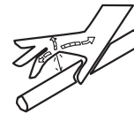
Hydraulic Fluid Penetration
