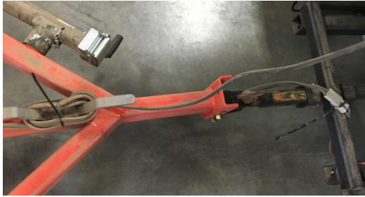
3. Connect hitch to tow vehicle. Adjust hitch as necessary to level roller frame. Best performance is achieved with roller frame level or hitch slightly up.
