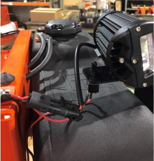
3. Connect wiring to the lights. Wiring can run in back of the machine at the top. Zip tie the wiring to the bar at the back of the machine. Put the toggle switch in the switch tab.
