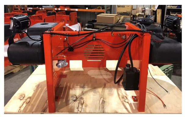
4. Fasten the fuse to the positive on the battery and black to the negative on the battery.
