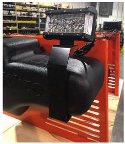
2. Bolt the lights to the light brackets. Bolt the switch tab under the light over the battery side for the toggle switch.
