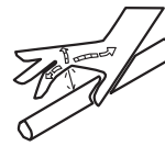
Hydraulic Fluid Penetration
